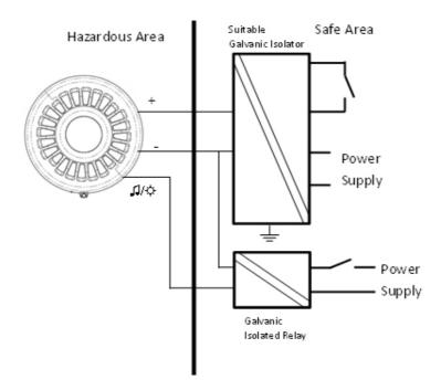
End of line monitoring is applicable to the Sounder Product. For this to function correctly, the resistor must be connected between the IN+ terminal and the Sounder Negative Supply. A suitable Zener Barrier which can allow reverse polarity monitoring to take place and a fire panel compatible with Intrinsically Safe products must also be used.
