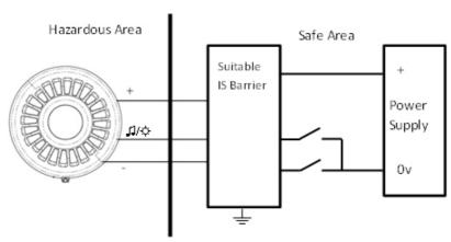
Switching between return paths will enable either Sounder or Beacon, alternately, both the paths could be activated to power both sections toaether.
