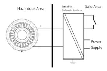
As with the Zener barriers, the Sounder and the Beacon can be triggered independently when using Galvanic Isolators, however an additional Intrinsically Safe relay is required to make the additional connection.
