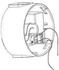
To locate Deep Base, unscrew mains module and use appropriate knock outs. Relocate mains module. Note - to use base box fittings only use the knockouts indicated. Do not remove label from deep base for alternative orientation.
